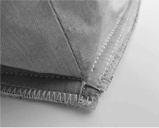
**16**, Finish the raw edges by serging or zigzag stitching around the quilted bottom.
